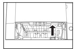
After you have removed the paper jam, replace the lower feed cover.
